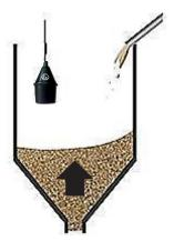
When the silo fills up, the level sensor is suspended vertically.
