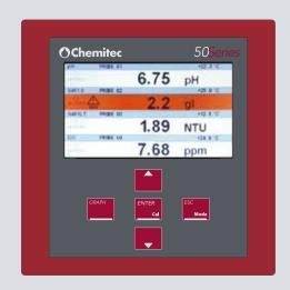
Complete and flexible system for a wide range of applications in water treatment with easy to use software and automatic recognition of sensors: available in three configurations, up to two (2), four (4) and eight (8) simultaneous measurements, freely selectable.
